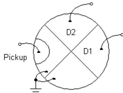
The drive forces are proportional to the square of the electric fields, so the frequency is doubled and the  $45^\circ$  phase shift becomes a  $90^\circ$  phase shift in the force. This combines with the  $90^\circ$  electrode orientation for the rotational force.
