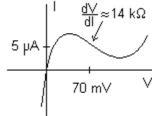
If the negative resistance ( $R_n$ ) is arranged to be in parallel with an LC circuit, it can cancel any positive resistance ( $R_Q$ ) associated with losses in the LC circuit and lead to exponential growth of oscillation instead of decay. The oscillations grow until the average negative resistance (averaged over the I-V curve) balances the regular dissipation, effectively regulating itself with  $R = \infty$ . This is typically 50 mVpp, depending on the details of the circuit
