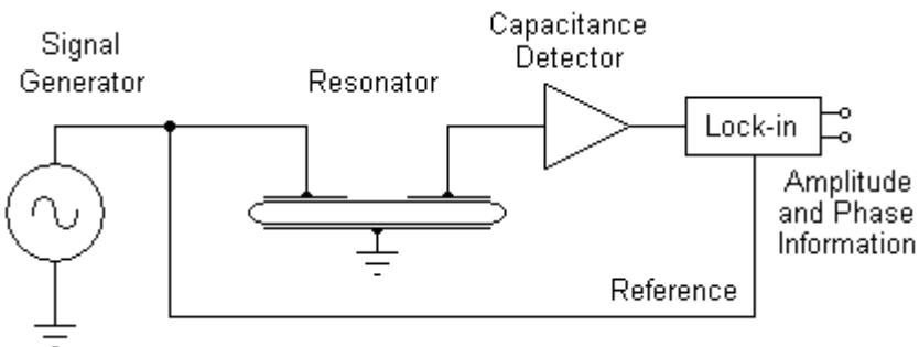
The goal is to detect film thickness sloshing inside of a resonating chamber. A signal generator applies an electric field of about  $10^6 \frac{V}{m}$  to the film on two opposite surfaces inside one capacitor of the resonator. Changes in a second capacitance are converted to a voltage and detected with a lock-in referenced to the drive.
