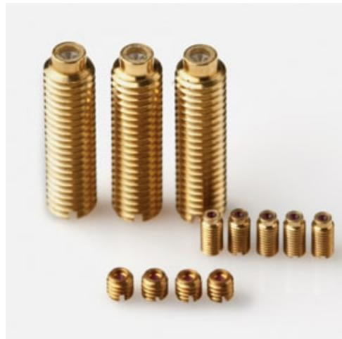
**Figure A.6:** A jewel bearing is a plain bearing in which a metal spindle turns inside a jewel-lined pivot hole. The image above is the jewel bearings used to reduce the friction on the needles when the dipole was oscillating. The jewel model is VS-100, length of .250", a radius of .003/.004", jewel size of V1.25, and thread size of 5-40 UNS-2. [17]
